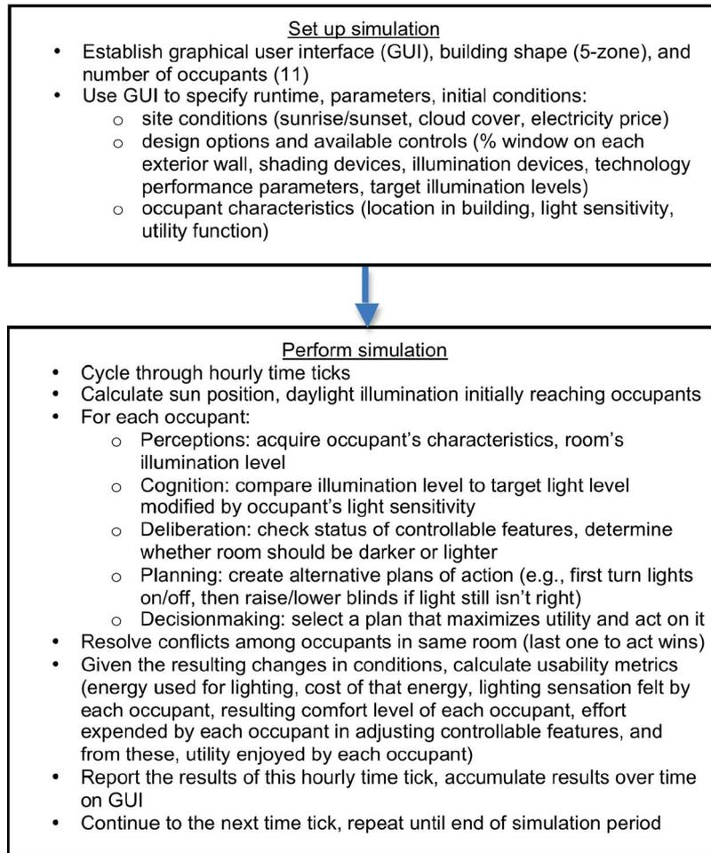
Fig. 5. Programming steps in the simulation model.
