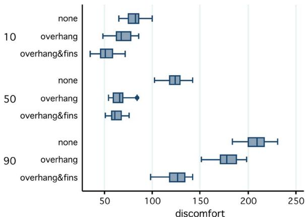
Fig. 9. Interactions between window size and window treatment. Note that 40 simulations were performed for each of the nine window %/window treatment combinations, holding fixed the lighting type (portable), occupants' light sensitivity (normal), and preferences (traditional consumer) but varying the electricity price. Window sizes are 10%, 50%, and 90% of the wall area. Window treatments include none, overhangs, and overhangs and fins.
